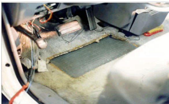
Floor-plate trap in the closed and open positions
