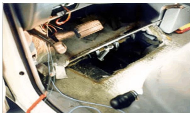
Floor-plate trap in the closed and open positions
