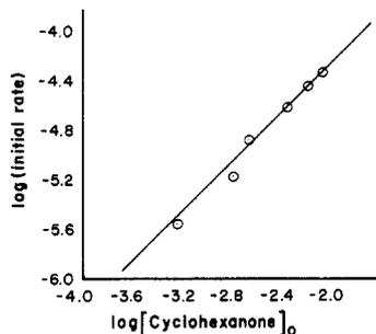
Figure 3. Plot of log (initial rate) against log [cyclohexanone]<sub>0</sub> with 0.10 M potassium phosphate for pH 7.90, [HSO<sub>3</sub><sup>-</sup>]<sub>0</sub> =  $8.7 \times 10^{-4}$  M, and [Py]<sub>0</sub> =  $1.60 \times 10^{-4}$  M at 25 °C. The slope is 0.98.
