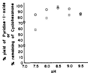
Figure 1. Percent yield of pyridine 1-oxide (○) with  $[py]_0 = [HSO_5^-]_0 = 2.93 \times 10^{-4}$  M, 0.15 M buffer potassium phosphate for pH 7.0–8.5 and sodium carbonate for pH 9.0–9.5, and cyclohexanone catalysis; also, percent remaining cyclohexanone (□) with  $[cyclohexanone]_0 = 0.0198$  M and  $[HSO_5^-]_0 = 0.0150$  M and the buffers as above, but no pyridine.
