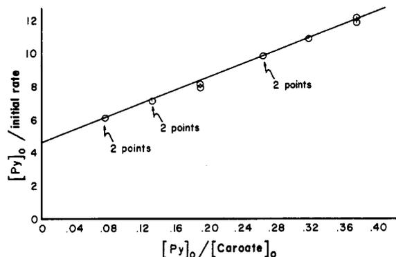
Figure 4. Typical plot of [Py]<sub>0</sub>/initial rate against [Py]<sub>0</sub>/[HSO<sub>5</sub><sup>-</sup>]<sub>0</sub>: [cyclohexanone]<sub>0</sub> = 6.13 × 10<sup>-3</sup> M, [HSO<sub>5</sub><sup>-</sup>]<sub>0</sub> = 8.26 × 10<sup>-4</sup> M, [Py]<sub>0</sub> from 6.19 × 10<sup>-5</sup> to 3.10 × 10<sup>-4</sup> M, and pH 7.90 with 0.1 M potassium phosphate buffer at 25 °C. The slope is 19.9, and the intercept is 4.63.
