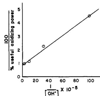
Figure 2. Plot of 100% useful oxidizing power against  $(1/[OH^-]) \times 10^5$  under conditions of  $[cyclohexanone]_0 = 0.0198$  M,  $[HSO_5^-]_0 = 0.0150$  M, no pyridine, and potassium phosphate buffer (0.12 M) for pH 7.0–8.5. The y intercept is 0.85 and the slope is 0.037.
