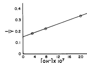
Figure 5. Typical plot of 1/γ vs. [OH<sup>-</sup>] for γ = slope/y intercept from plots such as Figure 4: [cyclohexanone]<sub>0</sub> = 3.07 × 10<sup>-3</sup> and 6.13 × 10<sup>-3</sup> M at pH values 7.50, 7.90, and 8.30. The slope is 9.19 × 10<sup>4</sup>, and intercept is 0.155.
