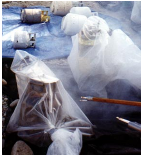
The top cylinders (on their side) contained ammonia. The bottom two are suspected HCl generators. They are wrapped in heavy clear plastic bags. pH test paper is being used to monitor their discharge.
