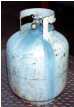
commonly encountered blue stain on clandestine lab cylinder, typically associated with ammonia
