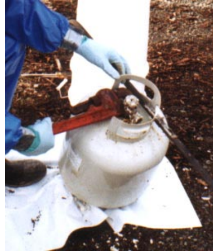
valve removal techniques (done only after generator pressure has been released)
