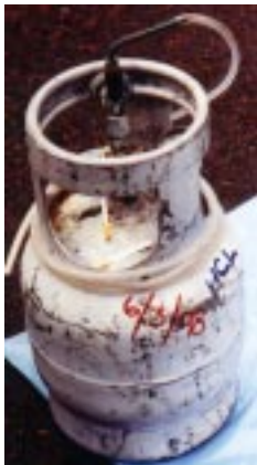
freon tank w/attached hose
