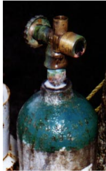
medical oxygen bottles (the manufacturer's valve has been illegally replaced with a POL brass propane tank valve)
