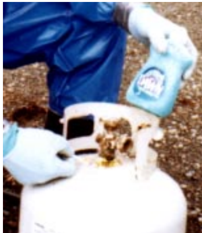
testing with soap for leaks around the valve neck
