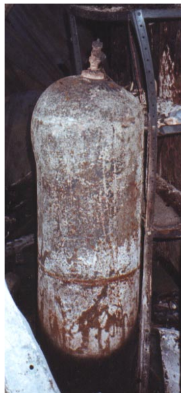
bulging cylinder that has been exposed to fire
