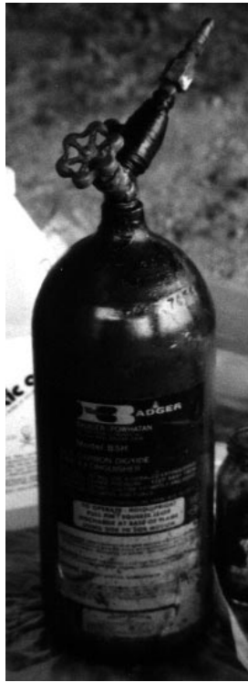
CO2 fire extinguisher with modified valve
