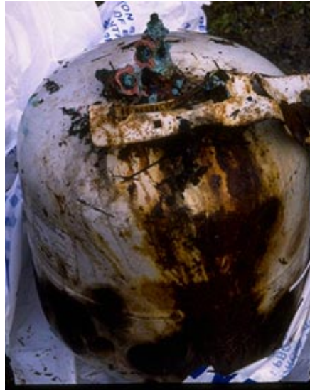
Burn marks on lower portion of tank are most likely caused by a torch. The collar at the top of the cylinder has been removed by the clandestine lab operator to provide better access to the valve ,which is also severely corroded
