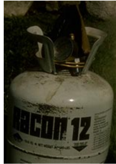
freon tank with home-made valve and hose connection
