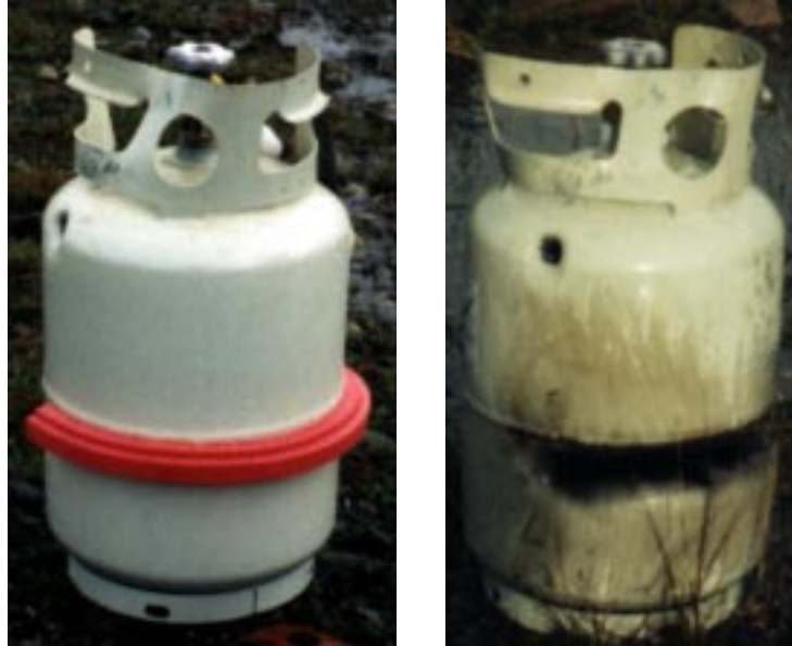
Shape charge applied to empty tank Before and after photos.
