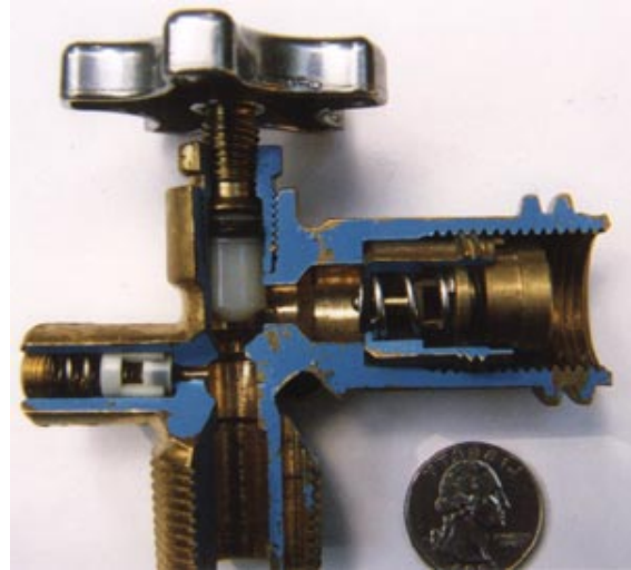
.....Type 1 valve, cutaway
