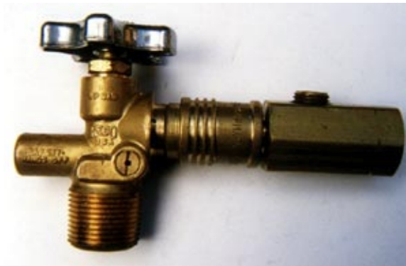
Type 2 valve with adaptor from hardware store that depresses internal fitting allowing propane to flow
