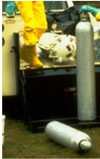
commercial HCl cylinder being loaded for transport
