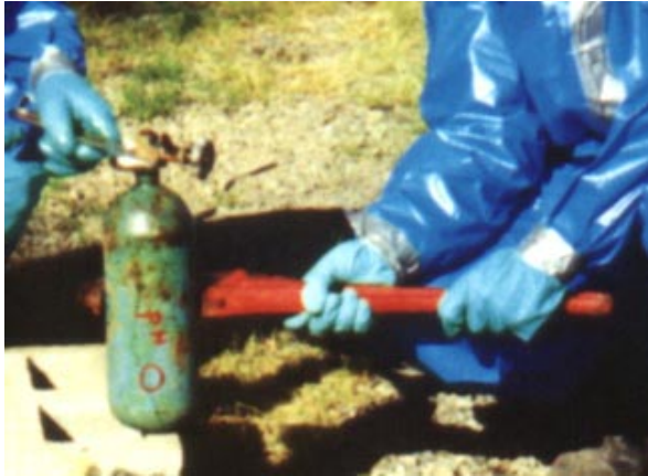
valve removal techniques (done only after generator pressure has been released)
