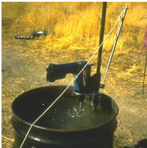
Remote drill setup and remote drilling under water. (A parts list of the hardware used for this setup is in earlier reports prepared for Ecology on NH 3 cylinders. Contact them for a copy.)
