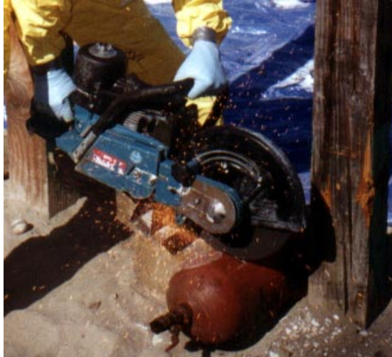
chop or 'cut' saw being used, note the sparks being produced
