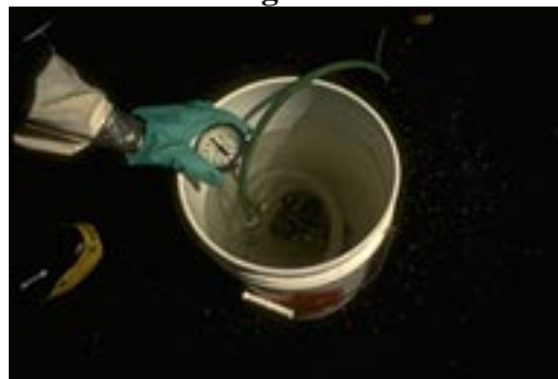
sparging into water while monitoring temperature (A parts list of the hardware used for this sparging setup is in earlier reports prepared for Ecology on NH 3 cylinders. Contact them for a copy.)
