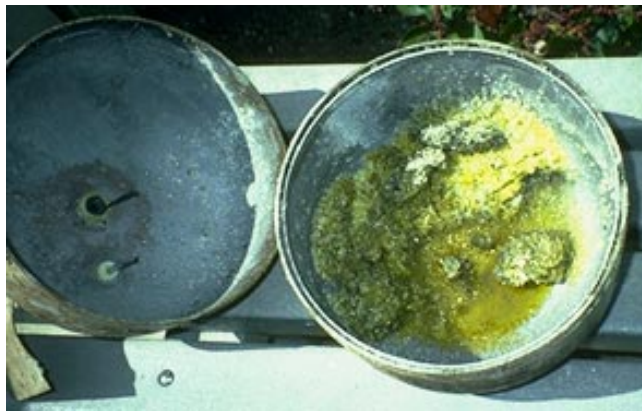
waste material described as “dirty wet rock salt” found in 5 gallon propane tank HCl generator
