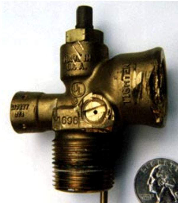
.....Brass POL propane valve (note the tool marks, indicating it has been improperly removed .....from a cylinder
