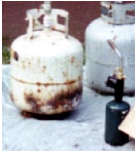
Burn marks on HCl generator created with propane torch.
