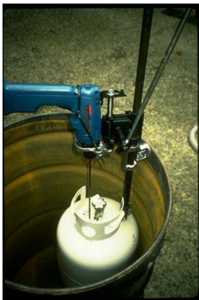
Remote drill setup and remote drilling under water. (A parts list of the hardware used for this setup is in earlier reports prepared for Ecology on NH 3 cylinders. Contact them for a copy.)
