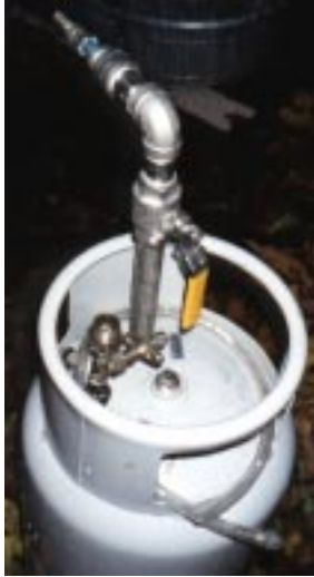
..home-made stainless steel valve assembly on 10 gallon propane tank
