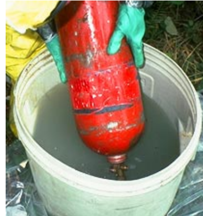
nearly spent HCl generator being manipulated by hand to try and clear blockage in the valve and neck from "sludge" in the generator
