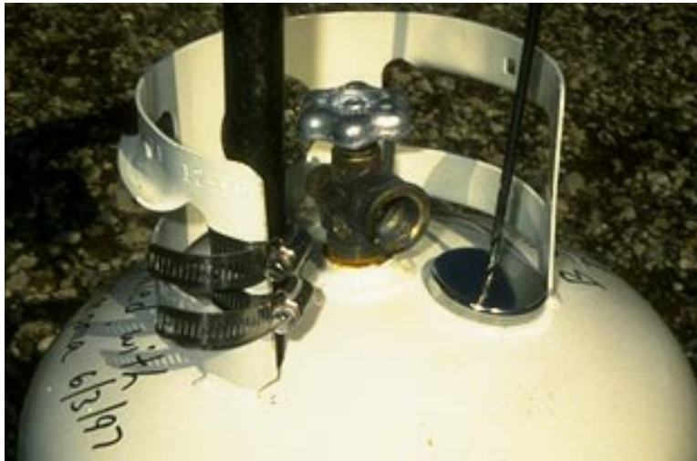
Close up of remote drilling hardware. Note circular magnet to keep drill bit from “walking.”
