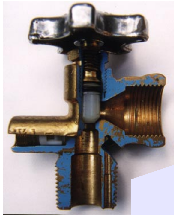
Brass POL valve, cutaway
